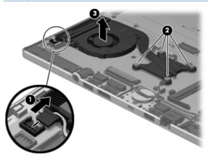
**NOTE:** The thermal material must be thoroughly cleaned from the surfaces of the fan/heat sink assembly and the processor each time the fan/heat sink assembly is removed. Replacement thermal material is included with the fan/heat sink assembly and system board spare part kits. Thermal paste is used on the processor (1) and the section of the fan/heat sink assembly (2) that services it.
