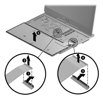
Reverse this procedure to install the keyboard.
