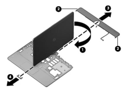
Reverse this procedure to install the hinge cover and hinge cap.
