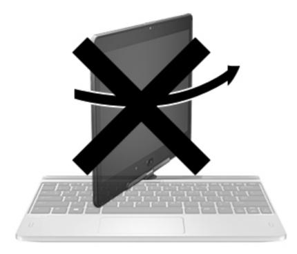
**CAUTION:** To prevent damage to the display hinges, when in notebook configuration, do not rotate the display counterclockwise, and do not force the rotating action.
