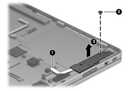
Reverse this procedure to install the button board.
