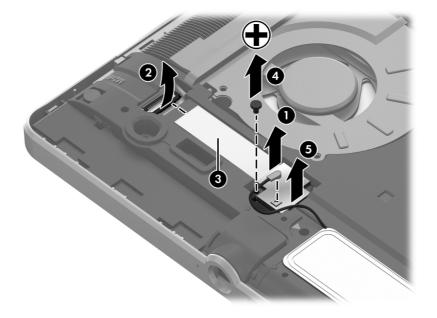
Reverse this procedure to install the NFC board.
