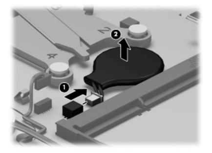
**3.** Remove the RTC battery.
