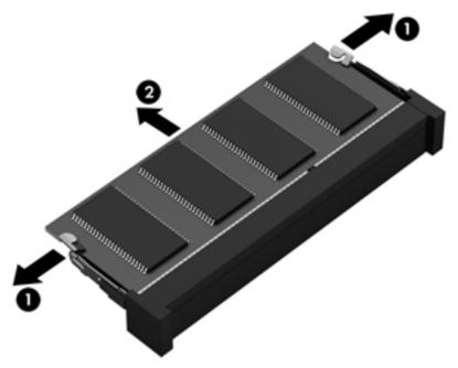
To protect a memory module after removal, place it in an electrostatic-safe container.
