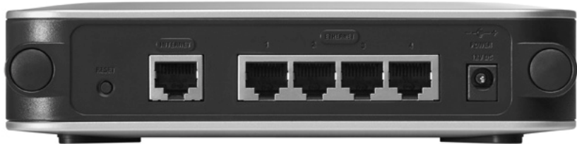
Figure 2. Cisco RVS4000 Gigabit Security Router Port Connections
